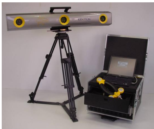
Fig. 7 Mobile co-ordinate measurement machine
